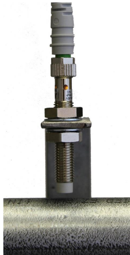
Too low – light is on with no hanger.
