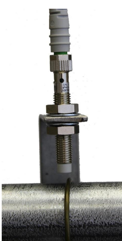
Too high - light is off with hanger in place.
